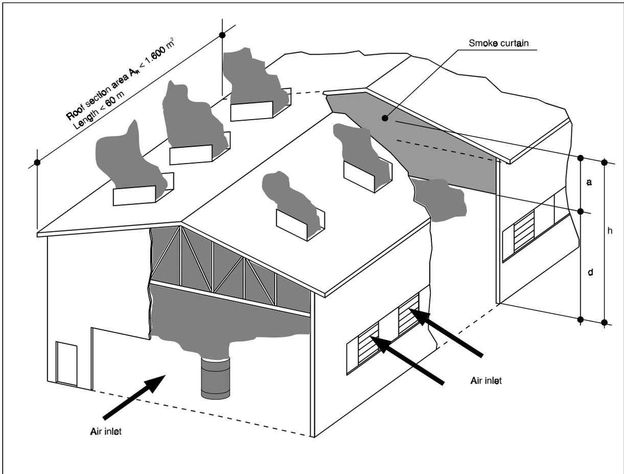
**Figures 1a, b:** Operating principle of Natural Smoke and Heat Exhaust Systems
