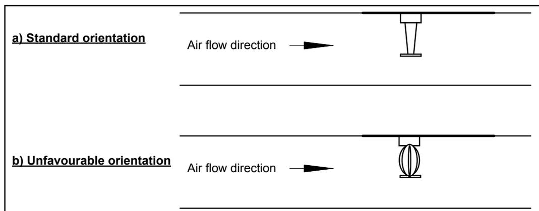
Test all other sprinklers where the influence other than yoke arm shadows can be encountered in different orientations to establish that the total angle of acceptable operation is  $\geq 256^\circ$ .
