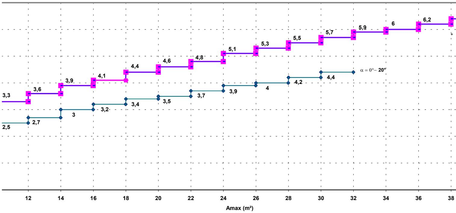
**Figure. 7: Maximum gap between a point on the ceiling and a smoke detector as defined in EN 54-7**
