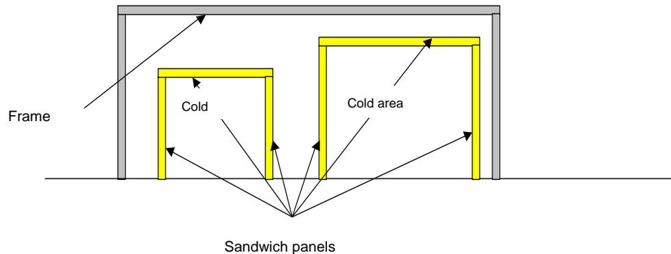
**Figure 2: internal sandwich panel systems**
