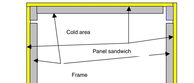
Figure 1 : external sandwich panel systems
